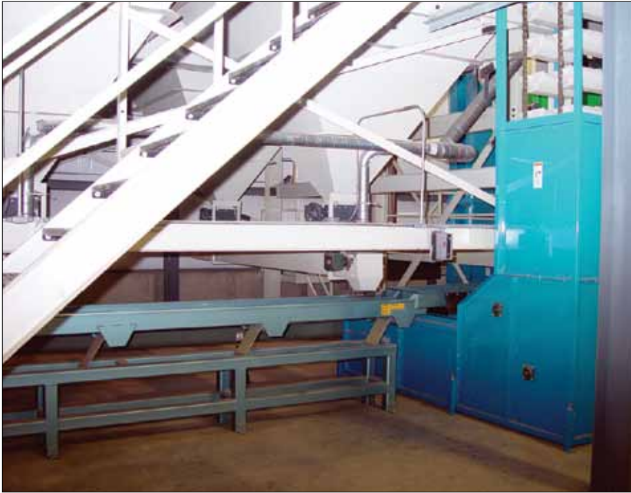
A Universal Industries DAKOSA™ split-bucket receives seed from a Forsberg split trough vibratory conveyor.
