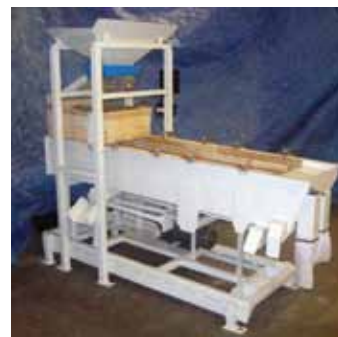
Popp Engineering continuous flow large sample seed corn sizer.
