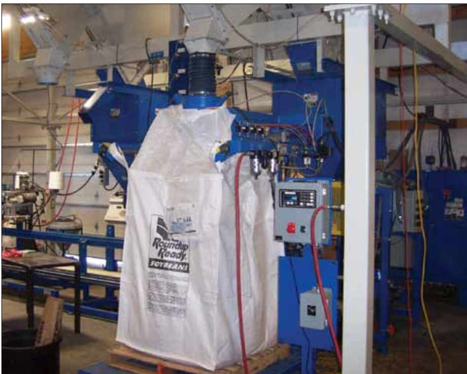
Filling spout-top bulk bag. Single-unit heat seal closer and bag stitcher in the background.
